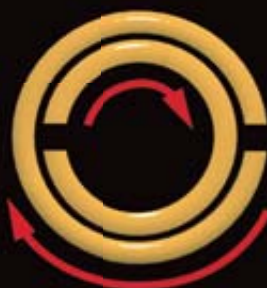
Circular currents flow in split-ring resonators (SRRs).
