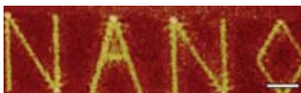
THIN LAYER OF SILVER acts like a superlens over very short distances. Here the word "NANO" is imaged with a focused ion beam (left), optically without a superlens (middle) and optically with
