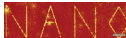
a 35-nanometer layer of silver in place (right). Scale bar is 2,000 nanometers long. With the superlens, the resolution is finer than the 365-nanometer wavelength of the light used.
